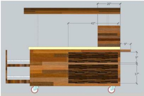
Mobile Kiosk Rear Elevation
