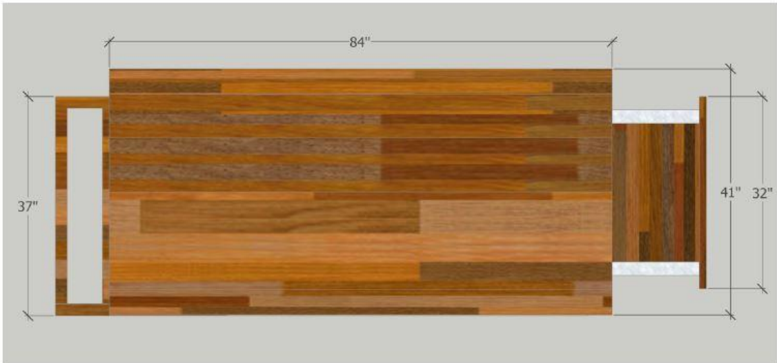
Mobile Kiosk Top Elevation
